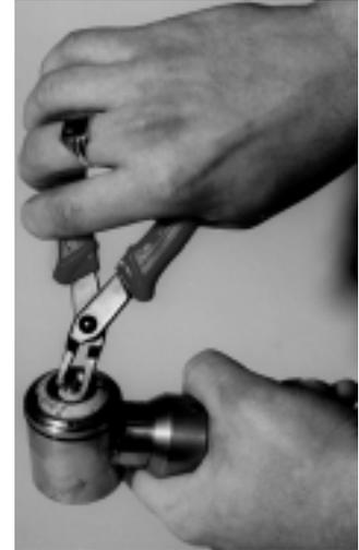
5. Press a new Electrode Assembly carefully but firmly over the contact tube until it is fully home and central. Use the handle of the Nozzle Tool which has been prepared for this purpose. **THIS IS VERY IMPORTANT !** If the Electrode is not pressed fully home onto the Contact Tube, the Swirl Bush may be partly crushed by the Nozzle, and will interfere with the airflow.
